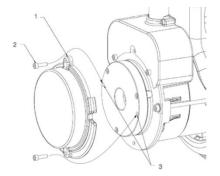
1. Braking cover 2. End cap bolt 3. Separating hole
