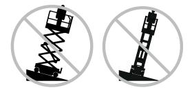
Do not use the tilt alarm as a horizontal indicator. The tilt alarm on the platform will ring only when the machine is heavily tilted.
