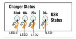
1.3 The battery charging procedure displayed on LED is shown as follows:
