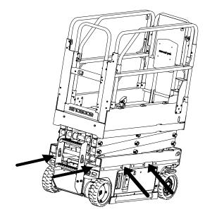
The forklift fork is aligned to the position of forklift slot.
